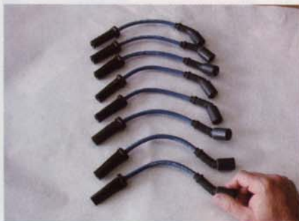
We first wanted to see if we could improve the truck's power by simply replacing the factory plug wires with Granatelli Hi-Performance wires. They offer high-temperature silicone boots and an 8mm jacket with a fiberglass-reinforced braid to withstand engine temperatures to 500°F.
