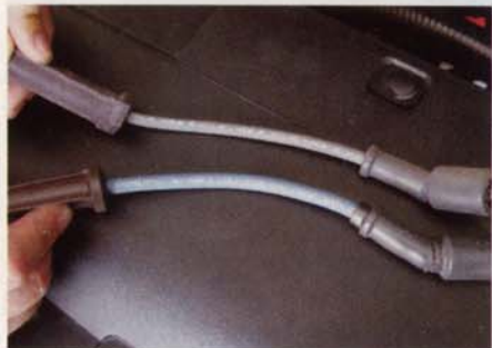
The stock AC Delco wire is composed of 7.5mm material (shown upper), compared to the 8mm-thick Granatelli wires (shown lower).
