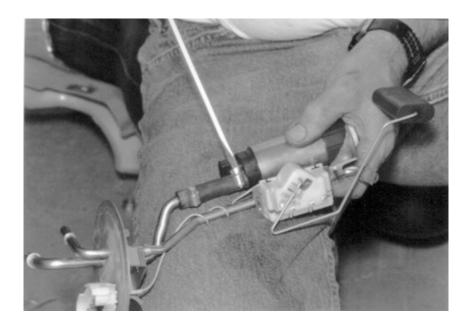
8. Hook up the electrical wires using the crimp connectors supplied with the fuel pump.
