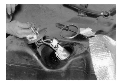
4. Pry the fuel filter off the fuel pump noting which way the large part of the filter is pointing.
