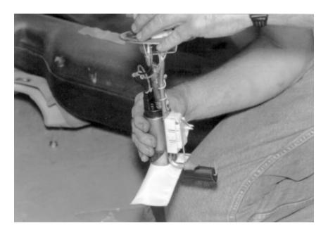
10. Slide the fuel pump into the fuel tank and make sure the O ring seal is in the O ring groove. Tighten the large nut that holds the fuel pump in the tank and Install the fuel tank on the car. The plastic safety clips that lock the fuel lines to the fuel tank are inexpensive and at your Ford dealer if needed.
