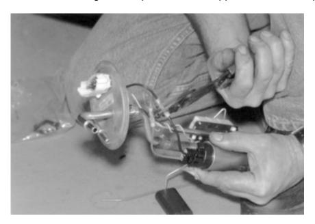
9. Push the fuel filter securely on the fuel pump. Make sure it is positioned in the proper direction.
