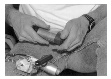
7. Slide the rubber hose and hose clamps over the fuel pump outlet. Slide the fuel pump into its mount and tighten the hose clamps. On the Thunderbird this hose will need to be shortened and the bend straightened out.
