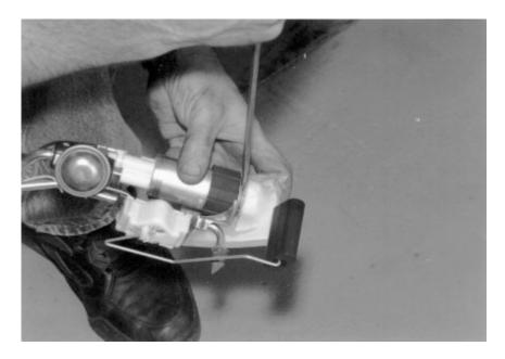
5. Pull the production fuel pump up and slide it out of its mount. Cut the electrical wires and remove the fuel pump.
