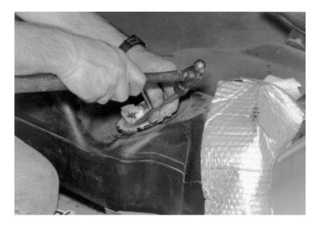
3. Remove the fuel pump/fuel level assembly.
