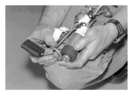
6. Slide the bottom rubber over the new fuel pump.
