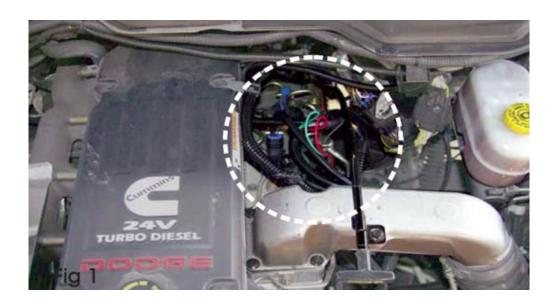
3. Disconnect the map sensor by gently lifting on the locking tab on the connector and remove the connector from the sensor. Plug the corresponding Big G connector into the sensor and plug the factory connector into the Big G harness. Make sure the plugs are completely locked together and you can confirm that the locking tabs on both connectors have been properly locked down.
