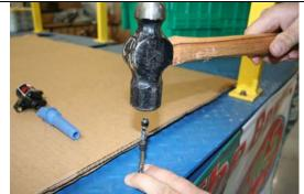
Gently tap the top of the either terminal end with a ball peen hammer as shown. This will allow to terminal ends to slightly compress closer to each other.
