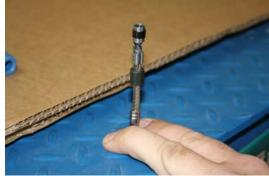
Stand the Stainless steel rope up on end as pictured - Note - This must be done on a hard surface.
