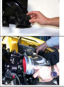
9. Place the supplied silicon sleeve around the oval throttle body side of the Granatelli intake tube.
