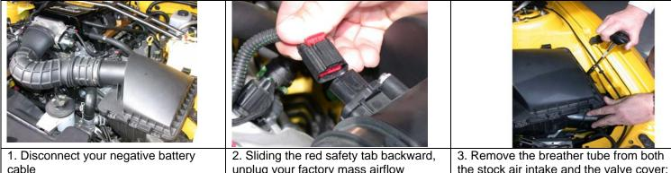
unplug your factory mass airflow sensor. Depress the black and slide the connector from the sensor itself.
