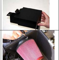
12. Place the air filter clamp over the air intake tube, followed by the air filter itself. Use the clamp to tighten the filter into place.
