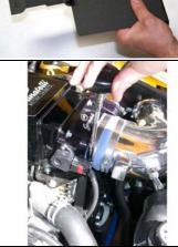
11. Place the Granatelli air intake assembly into the approximate location in the engine bay with the air filter end inside the heat shield area. Slide the silicon sleeve over the throttle body. Use the hose clamp to tighten the air intake tube securely to throttle body. Note: Make sure hose clamps go in the same direction to insure a cleaner look.
